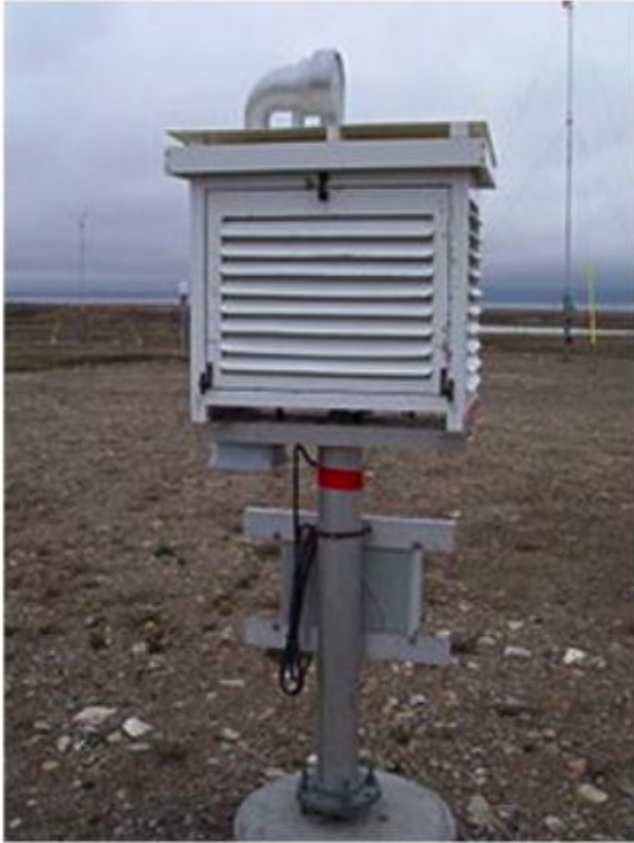
Exterior of a Stevenson screen
