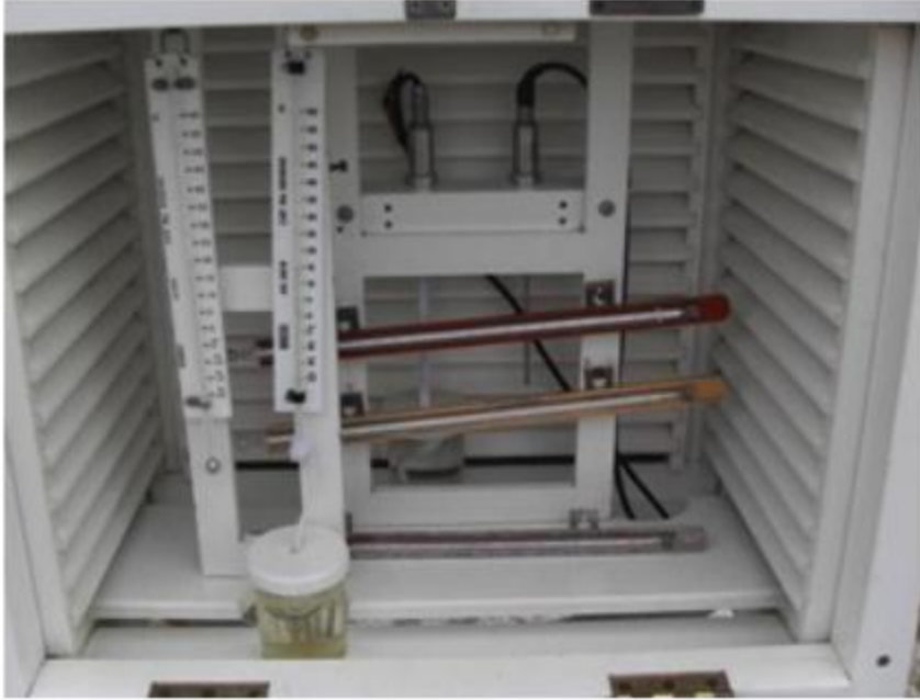
Interior of a Stevenson screen
